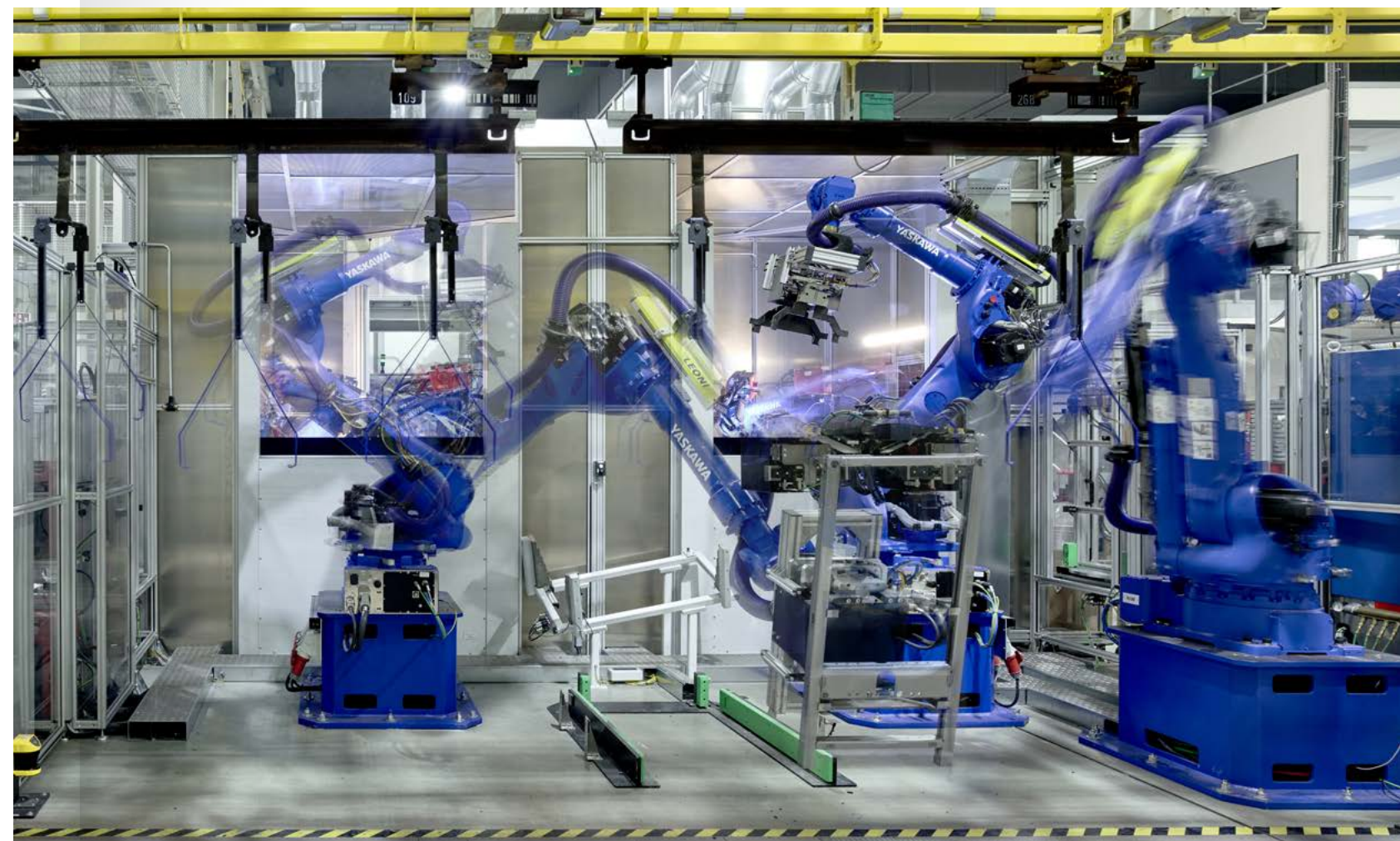
1 Automated production of Geberit installation elements. Photo credit: Geberit AG.
